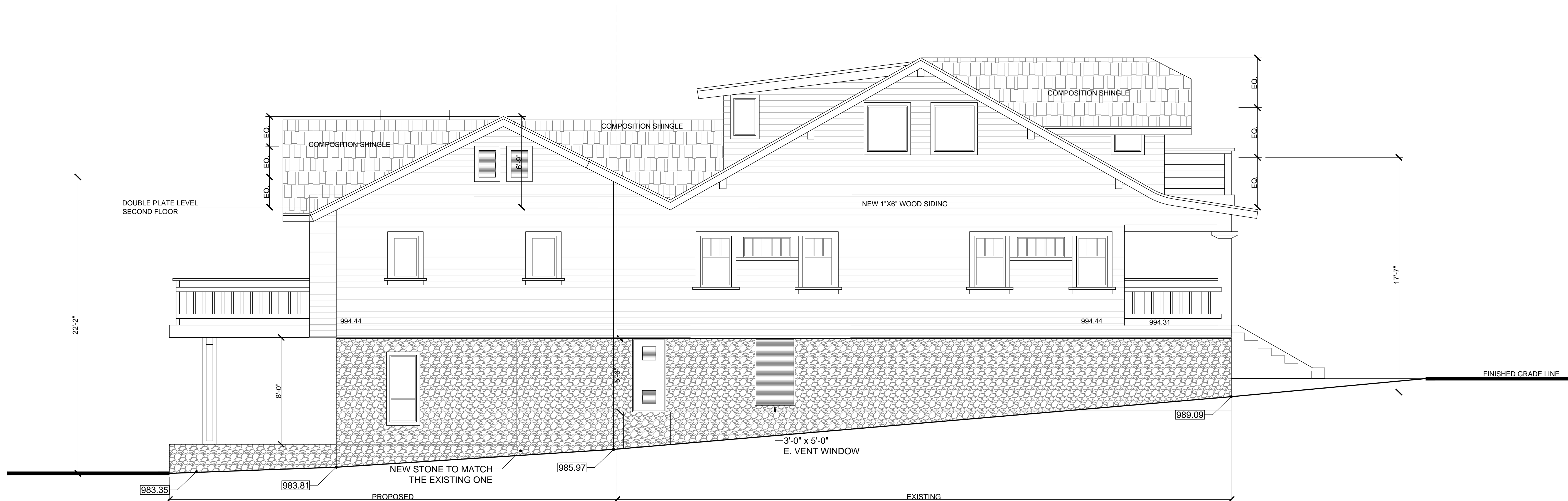
PROPOSED EAST ELEVATION SCALE 1/4" : 1'-0" EXISTING EAST ELEVATION AREA = 571 SQ.FT. PROPOSED ADDITION EAST ELEVATION AREA = 970 SQ.FT.
