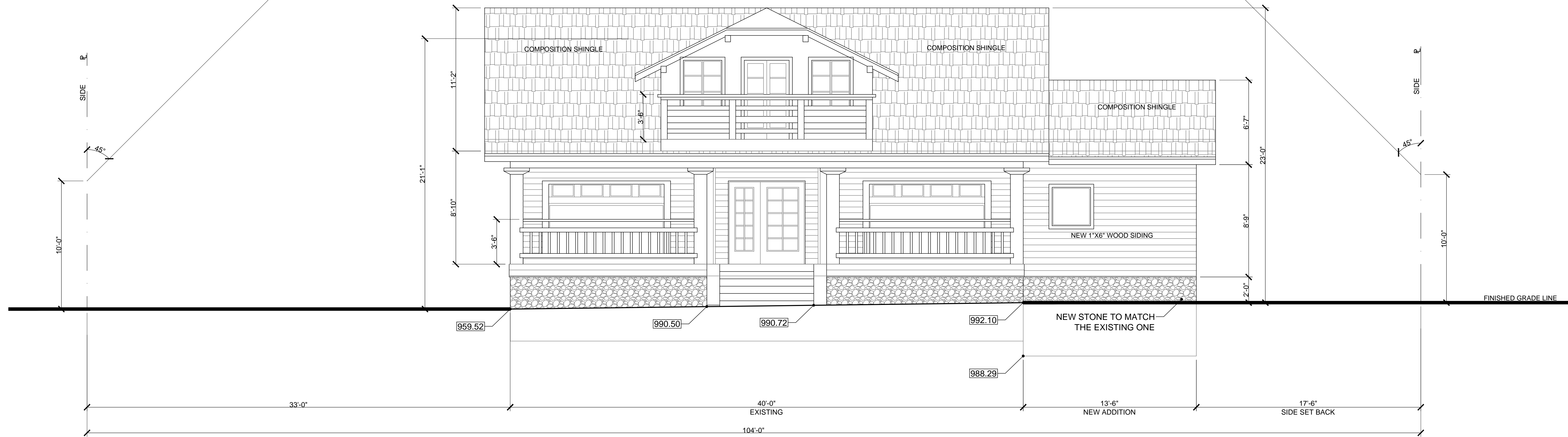
EXISTING & PROPOSED NORTH ELEVATION (FRONT) SCALE \frac{1}{4}" : 1'-0" EXISTING NORTH ELEVATION AREA = 613 SQ.FT. PROPOSED ADDITION NORTH ELEVATION AREA = 147 SQ.FT.
