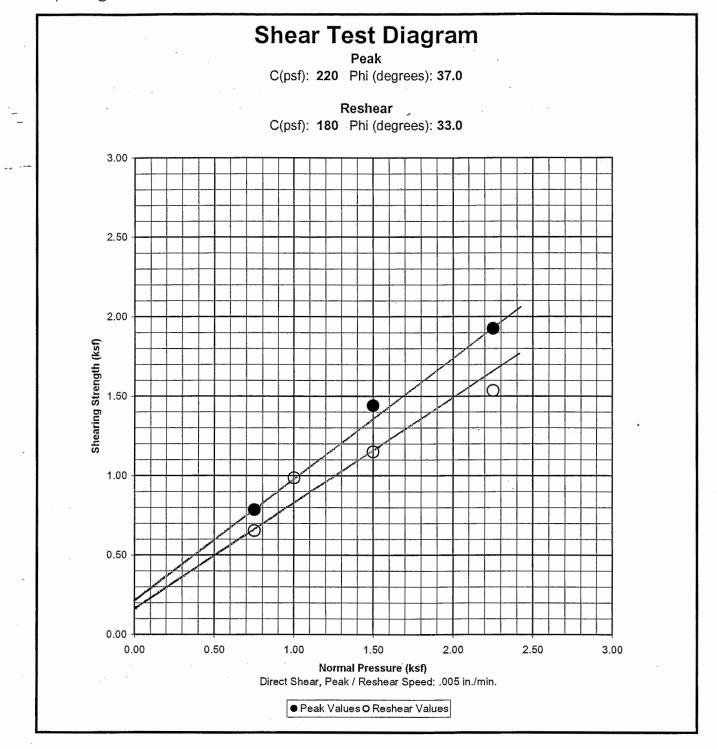
Sample **Remolded** to 90% Relative Density, saturated. Rem Dry Den = 106.2 PCF
