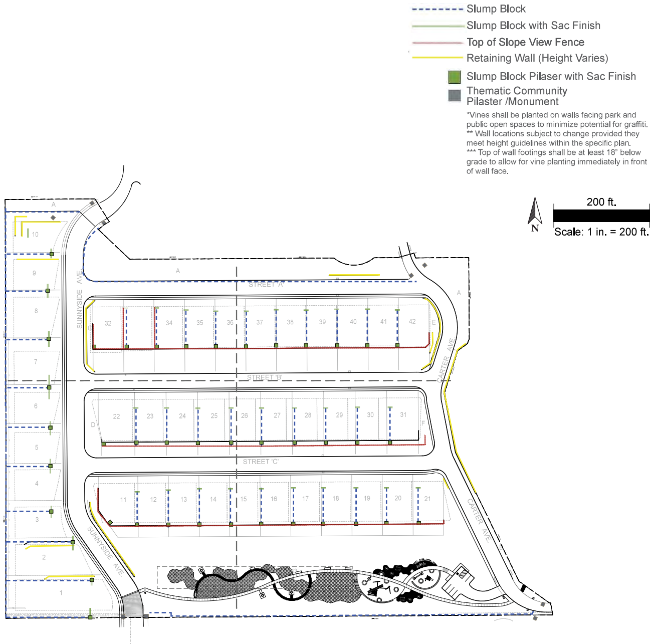
Figure 3-11a: Wall and Fence Plan Note: Refer to Appendix 3A, Figure Enlargements for plan details.
