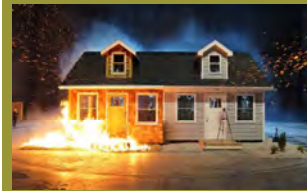
Figure 2b Embers impacting a building: left side with combustible (wood) and the right with noncombustible (rock) mulch.
