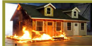
Figure 1 – Creating and maintaining home ignition zones (defensible space) around your property are proven ways to reduce risks of property damage during a wildfire, as tests at the IBHS Research Center have shown.
