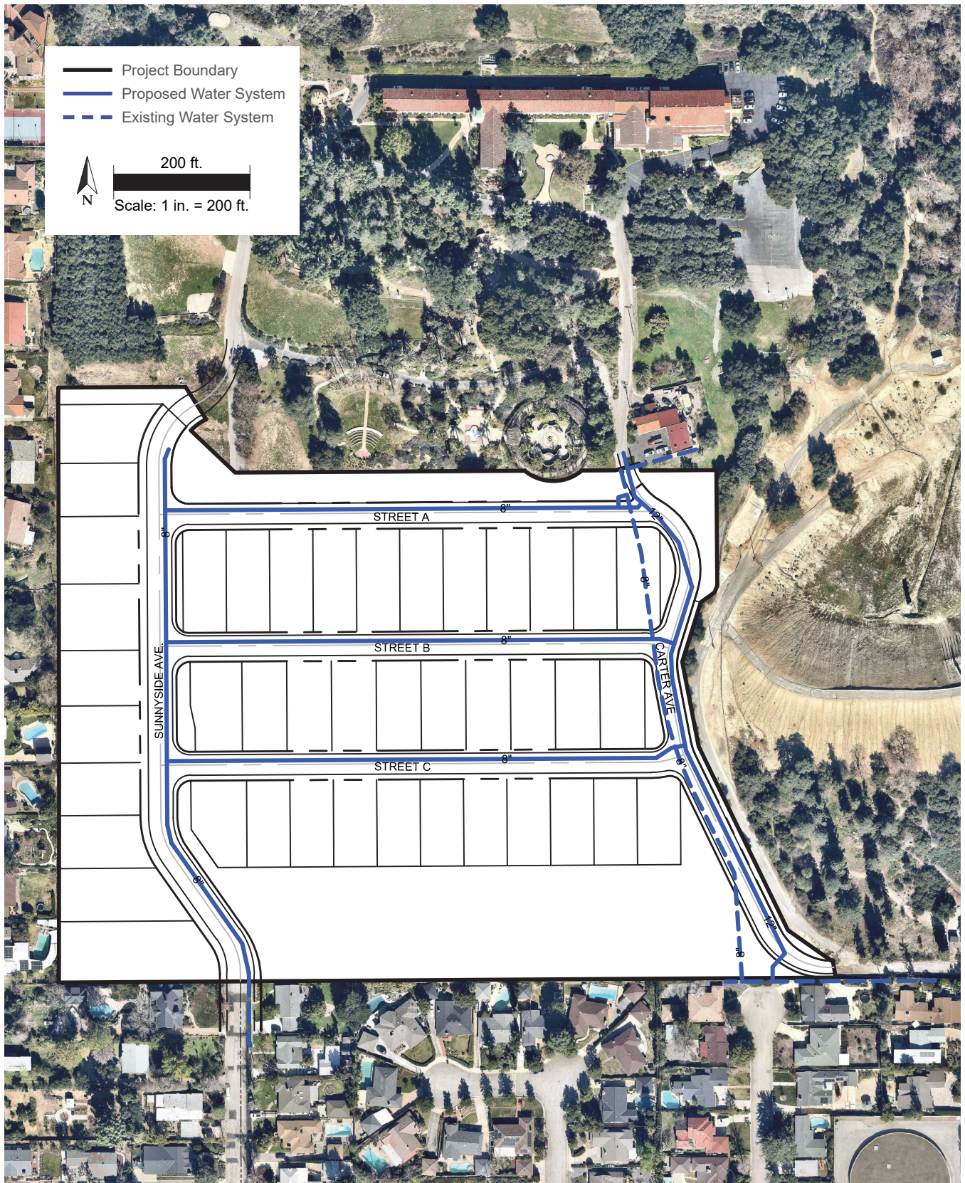
Figure 4-7: Existing and Proposed Water System
