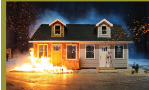
Figure 2b Embers impacting a building; left side with combustible (wood) mulch and the right side with noncombustible (rock) mulch.
