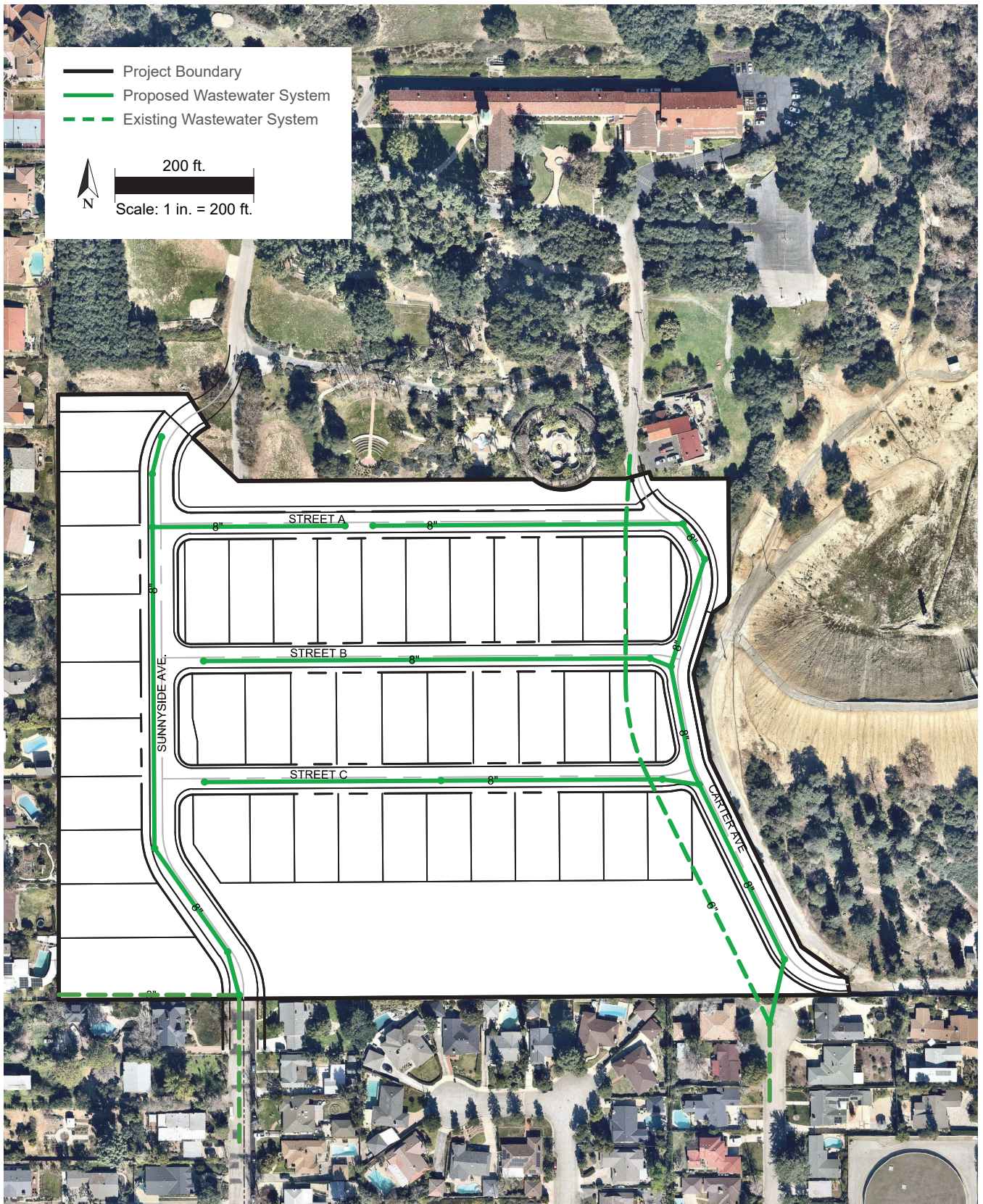
Figure 4-8: Existing and Proposed Wastewater System
