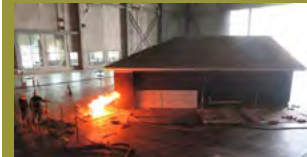
Figure 2a Experiments conducted at the IBHS Research Center to study the effectiveness of creating a noncombustible space around buildings.
