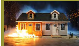
Figure 2b Embers impacting a building; left side with combustible (wood) mulch and the right side with noncombustible (rock) mulch.
