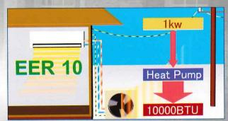
Heat pumps are more efficient than some other forms of heating because heat pumps do not actually create heat - they just move it from one place to another. For example, the output of an efficient 10 EER heat pump is triple that of an electric heater.
