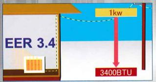
An electric heater converts electricity directly to heat, and if we assume that the heat loss is zero, the output from one kilowatt input is one kilowatt or 3,400 BTU and the EER is 3.4.
